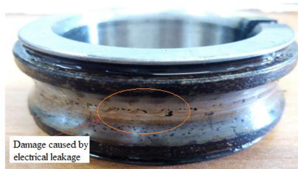
Figure 8- Destructive effects of the electric current leakage on the bearings
